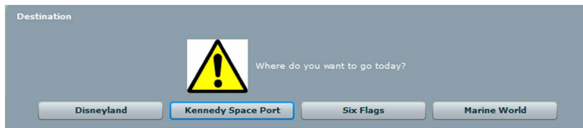
Figure 12.10 Pimped-out alert with a custom icon, custom button labels, and a default button
