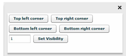
Figure 12.3 MoveWindow.mxml : clicking the buttons manipulates the x and y coordinates to reposition this pop-up.
